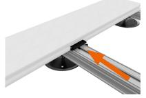
Insert the installation clips into the sub profile. Turn and push along the lower deck board edge. Clip may need to be tapped with a rubber mallet to secure firmly against the board
