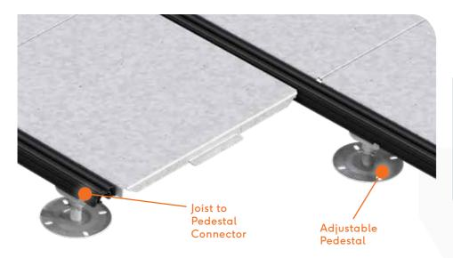
Rigid aluminium extruded joist rails for use as a support structure system to decking and paving. Raaft<sup>®</sup> joists are designed to be used on roof terraces, balconies and other external podium construction areas.
