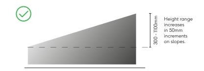
We can create planter panels with a sloped top edge. The shortest and highest height need to be in increments of 50mm.
