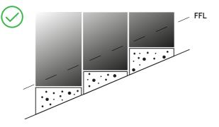
We can create level planters on a slope by stepping the concrete foundation and then changing the height of each planter panel to suit
